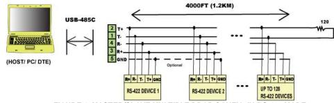
FIGURE 4: MASTER/SLAVE MULTIPLE DROP CONFIG. IN RS-422 MODE
