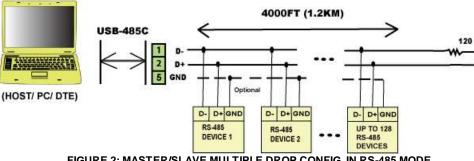
FIGURE 2: MASTER/SLAVE MULTIPLE DROP CONFIG. IN RS-485 MODE
