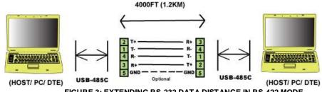
FIGURE 3: EXTENDING RS-232 DATA DISTANCE IN RS-422 MODE
